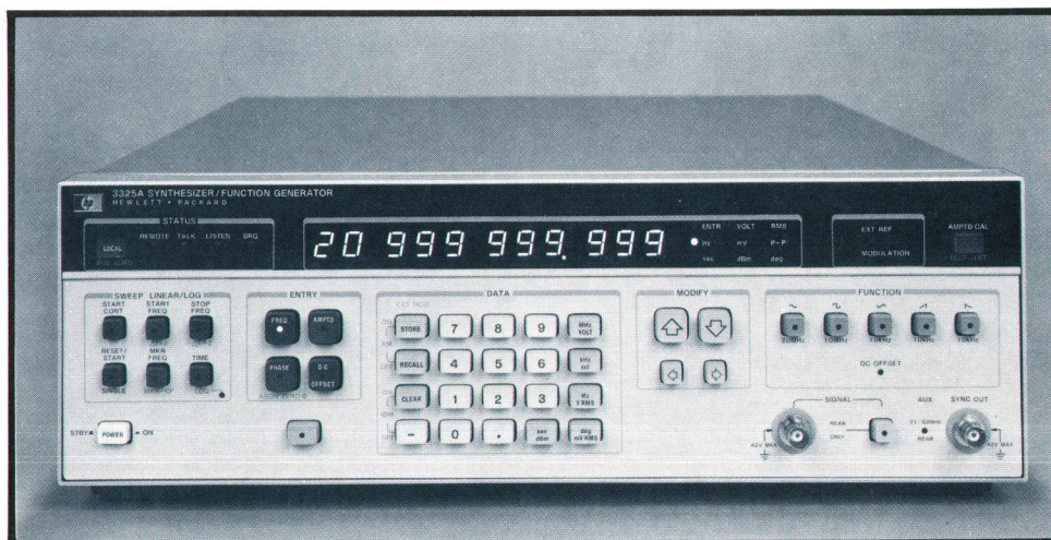
Fig. 1. Model 3325A Synthesizer/Function Generator produces waveforms with frequencies as low as 1 \mu Hz and as high as 21 MHz for sine waves (to 11 MHz for square waves and 11 kHz for triangles and ramps) with synthesizer accuracy. Output amplitude over the full frequency range is 1 mV to 10 V p-p into 50\Omega or, with an option, to 40V p-p into 500\Omega over a frequency range of 1 \mu Hz to 1 MHz. All necessary functions can be controlled through the HP interface bus as well as the front panel.
