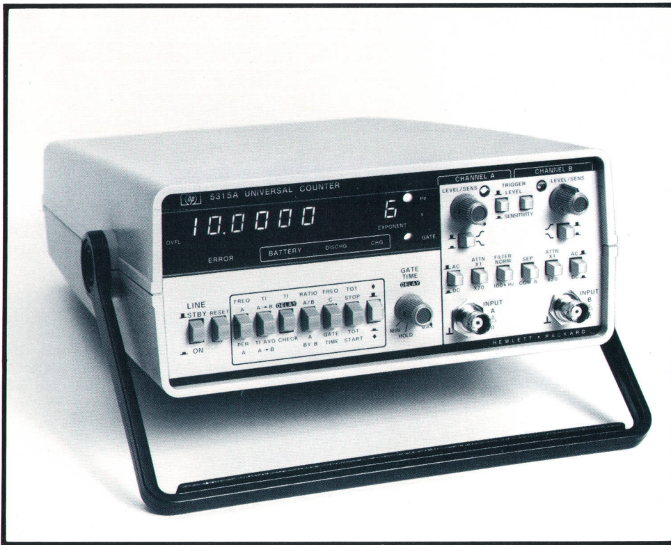
Fig. 1. Model 5315A Universal Counter measures frequency to 100 MHz and time intervals with 100-ns resolution. A reciprocal-taking two-channel instrument with a seven-digit display, it offers mid-range counter performance at a cost much lower than previous-generation counters. Shown here is the 5315A. The 5315B, the same instrument in a half-rack-width metal cabinet, offers exceptionally low radiated emissions.
